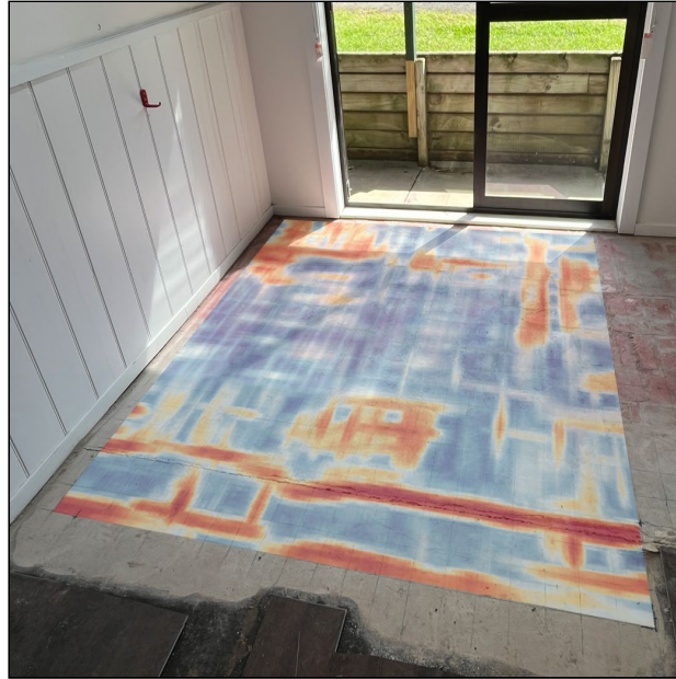
Depth slice: Subsurface layer (200-300mm)
