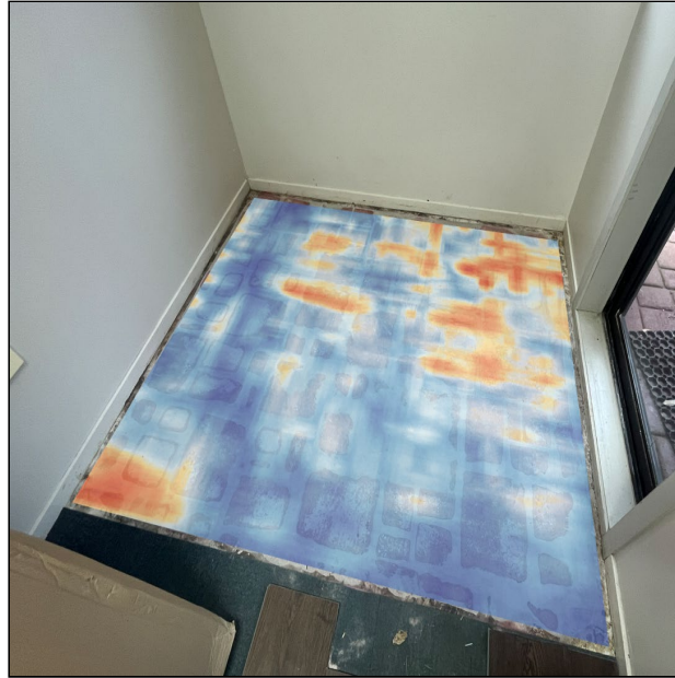
Depth slice: Subsurface layer (200-300mm)
