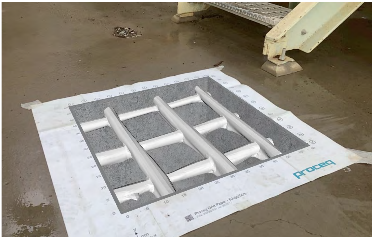
Figure 12: 3D visualisation of the scan data procured for Figure 9 above, confirming the overlap of the bars, including the placement of the east-to-west bars over the north-to-south bars (bars in place of scan over grid paper).
